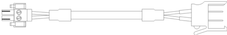
Figure 516 Layout of the FS-PDC-MB24-y power distribution cable
