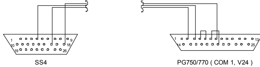
Fig. 6-7 SS4 at a PG750/770 ( COM1 ) via the RS 232 interface (the two jumpers for the PC are not required!)
