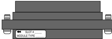
To remove the terminal block, loosen the upper and lower retaining screws. The terminal block will back away from the module as you remove the screws. When replacing the terminal block, torque the retaining screws to 0.46 Nm (4.1 in-lbs).
