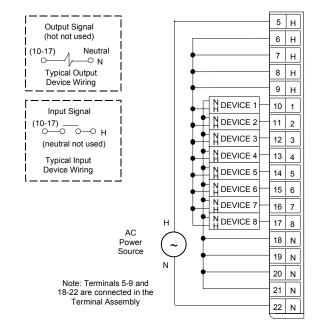
Connect a 115 volt AC source to one of the H terminals on the terminal strip. Connect neutral to an N terminal. All H terminals are internally bussed, as are all N terminals. Extra power terminals are for convenience. Depending on the physical layout and current loads, hot connections can be bussed together and made by one wire to the block or power source. Neutral connections can also be bussed together and made by one wire.
