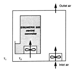
The air flow for removing lost heat is calculated from:
