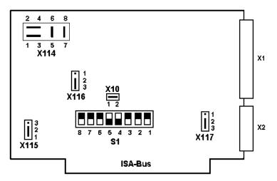
The factory settings of the jumpers and preset switch positions are shown in the figure. These default settings are indicated by "\*)" in the following table.
