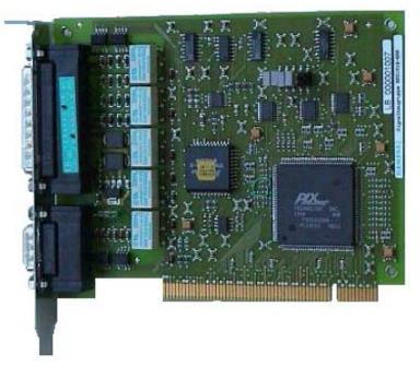
The signal module is plugged into the motherboard of the operator terminal PC. Check, whether a PCI slot is available.
