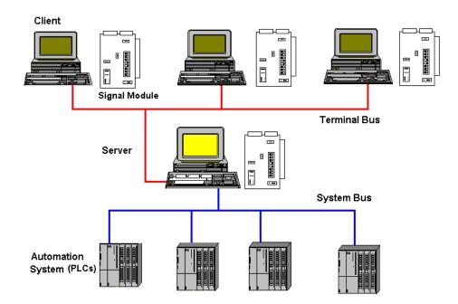
If the server operator station is to have multiple terminals (client operator stations), each terminal can be equipped with a signal module.
