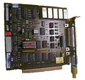
The signal module is plugged into the motherboard of the operator terminal PC. Check, whether an ISA slot is available. Note the addressing of the module to avoid address conflicts with other PC expansion cards. By default, the I/O address 180H is occupied by the signal module. For additional information, refer to the chapter "Addressing the ISA Bus Signal Module".
