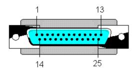
25-pin subminiature plug connector (pin connector with screw locking)
