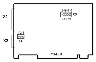
The factory settings of the jumpers and preset switch positions are shown in the figure.
