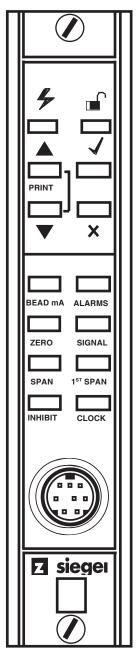
The front panel is fitted with a series of tactile pushbuttons for the operation of various functions, LEDs to provide rack power and communications status and a mini DIN socket for the connection of a serial printer, computer or an engineering key. The Engineering Key is used to unlock functions that can alter the operation of a control card.
