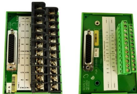
ET Blocks with screw terminals for lugged field wiring (left) and high-density "Euro" connectors for non-lugged field wiring (right)
