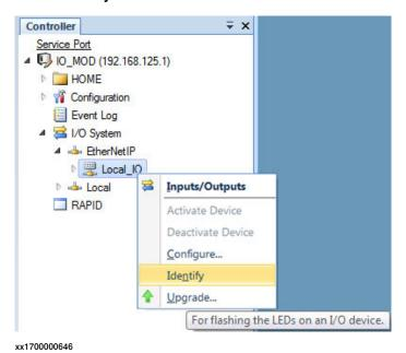
3 The PWR (Power) and NS (Network Status) LED of the physical base I/O device flashes to identify the I/O device in the controller.
