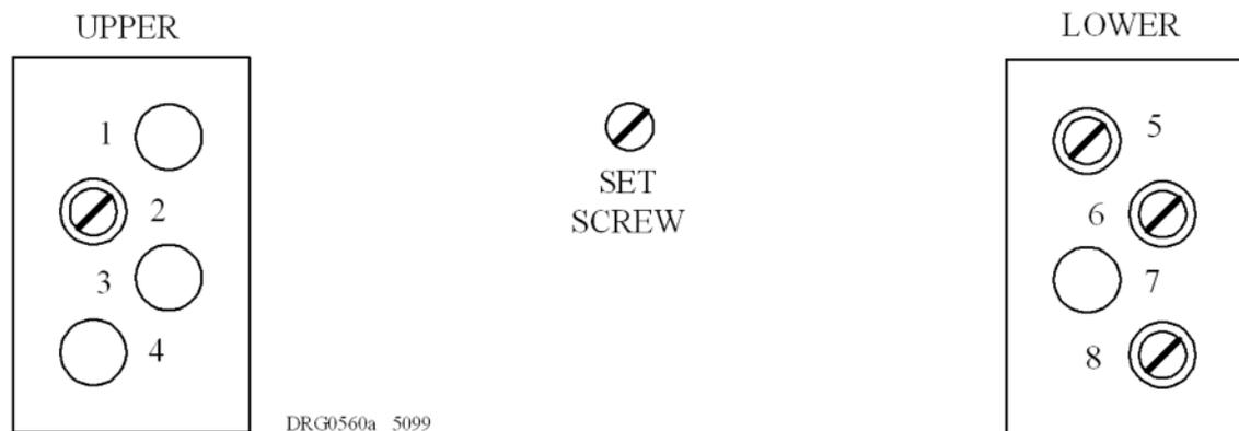
Figure 2-1 Chassis mechanical coding block configurations
